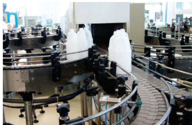
Plastic slat band conveyor transport water cans
