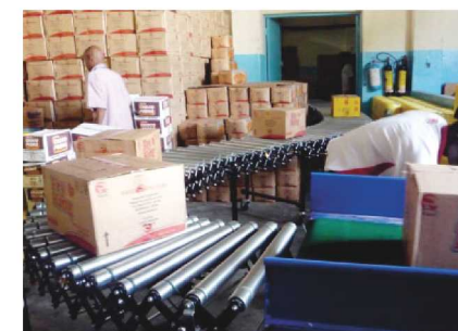
Combine with flexible conveyors to offloading cartons into warehouse
