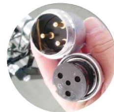
Supply power for additional sections by Air plug
