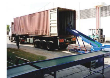
Combine with belt conveyors to loading bags from warehouse to containers
