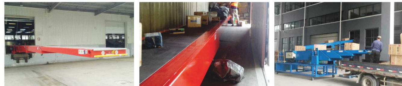
Telescopic Belt Conveyor applied in warehouse with docks
